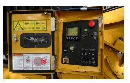
**VERMEER PLUS+1 CONTROL SYSTEM.** Offers four different speed options for more precise feed control. An optional wireless remote is available for enhanced operating efficiency
