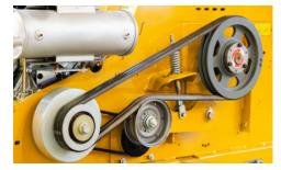
**THE CENTRIFUGAL CLUTCH**. Helps prevents belt-slip when engaging the clutch to minimize maintenance.
