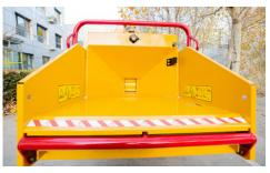
**THE LARGE INFEED OPENING.** 6 in x 8 in (15.2 cm x 20.3 cm) makes feeding irregular material efficient and minimizes the amount of saw cuts needed prior to feeding the chipper.
