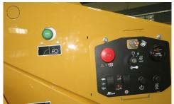
**THE CONTROL PANEL.** Fully weatherproof and contains a Siemens soft starter which helps protect the drum motor from overloading and voltage dips from the power grid.
